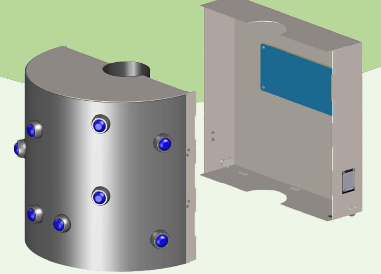
The device is mounted on the traffic light pole and consists of two interlocking parts. These parts are securely fastened around the pole, ensuring stability. Designed to be weather-resistant and durable, it can withstand various environmental conditions and potential damage.
